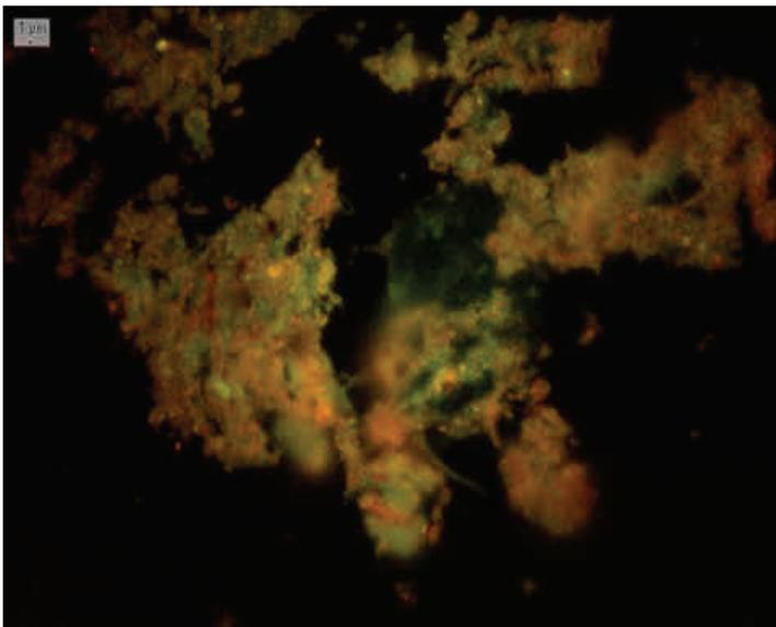
**Figure 6. Epifluorescence Optical Photomicrograph of 2-Week Saltwater Biofilm on Stainless Steel (2000X magnification, acridine orange stain)**
