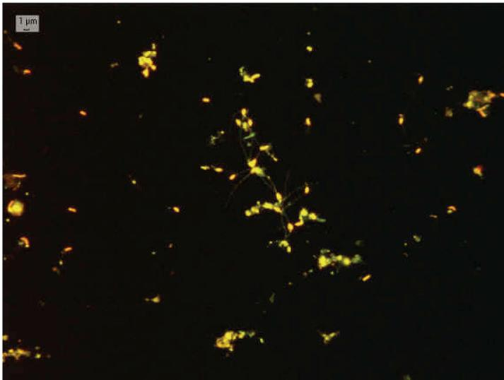
**graph of 2-Week Saltwater Biofilm on Stainless Steel after High-Shear Water Flush Cleaning (2000X magnification, acridene orange stain)**
