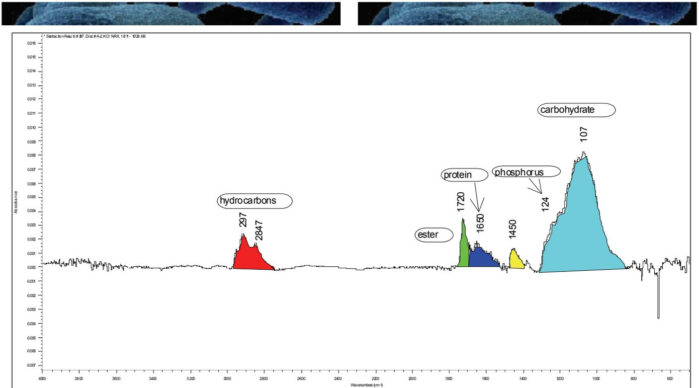
Figure 4. Fourier Transform Infrared Spectrum of Saltwater Biofilm
