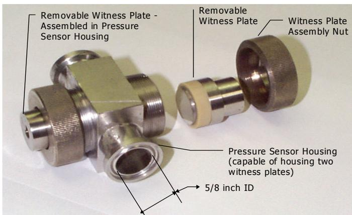
The fouling cell housing and discs are placed in a manufacturing process and removed after some specified time interval. The discs are taken out of the housing and then analyzed by a variety of techniques.
